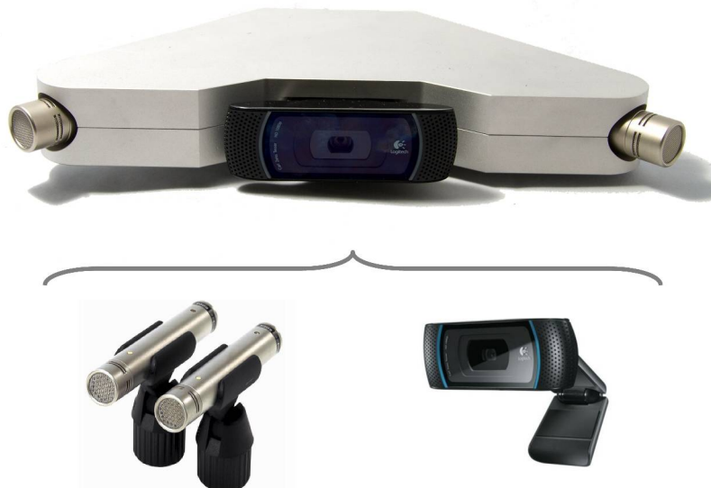
Figure 10 HD-Webcam and Stereo-Microphones integrated in a custom aluminium housing
