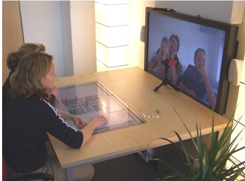
Figure 3 The Fraunhofer demonstration set up including a table top display and large screen video used to test the audio chain in the playing of a game remotely
