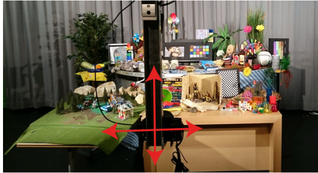
Figure 1: Camera and scene setup. The gantry system is partially visible in the foreground with the camera pointing to the scene.
