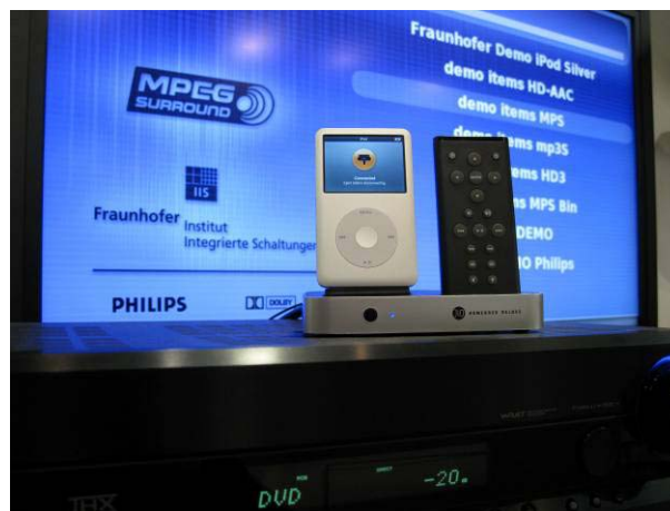
Figure 4: Prototype iPod Docking Station with MPEG Surround Decoder
