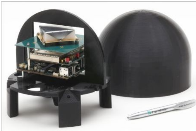
Figure 6. Smart Antenna build up with Open-GNSS Receiver
