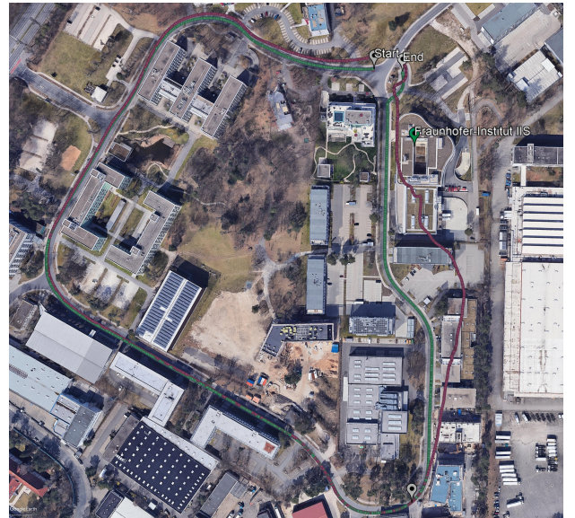
Fig. 3. The ideal trajectory from a reference system in green and the VDLL trajectory in orange of the test drive near the Fraunhofer IIS department, picture from Google Earth Pro.
