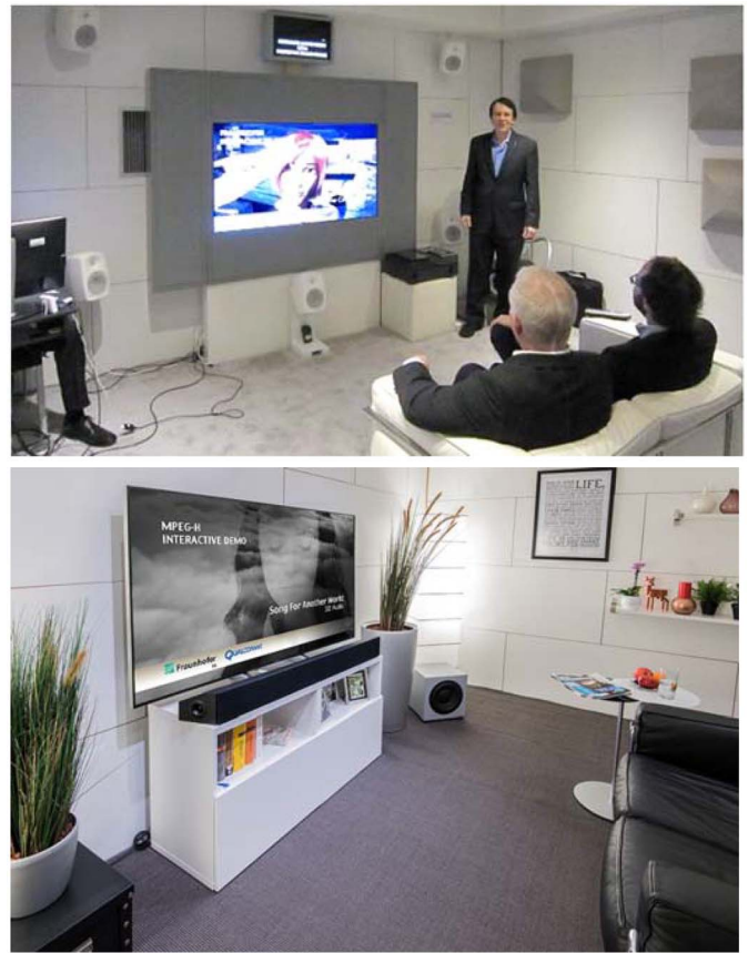
Fig. 46. 3D soundbar designs: (above) First-generation design. (below) Second-generation design. Wall-mounted loudspeakers in the left photo were used for discrete playback to simulate professional monitoring and enthusiast listening.
