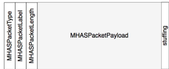
Fig. 31. MHAS packet structure.
